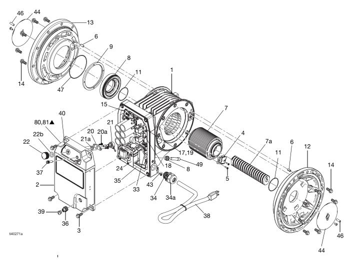
Fig. 20: Parts (Ordinary Locations model shown)
