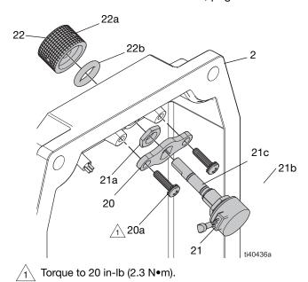
Fig. 9: Control Knob Assembly
