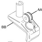
Fig. 5: Fan Press Tool
