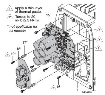
Fig. 10: Control Board and Filter Board
