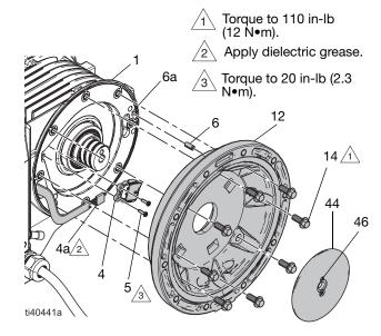
Fig. 11: Motor Sensor
