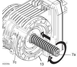
Fig. 18: Remove Rotor Greasing Tool
