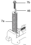
Fig. 14: Prepare the Shaft (7a) for Assembly
