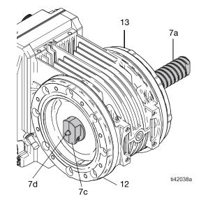
Fig. 17: Rotor Greasing Tool
