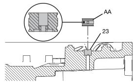
Fig. 6: Press Bushing on Motor Bearing
